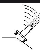
Moving the table on a sloping surface may cause the table to tip over, damage it or, more seriously, lead to injury. Take the necessary precautions.
